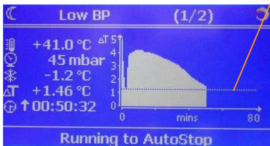
\Delta T trip point set, evaporator running to AutoStop
